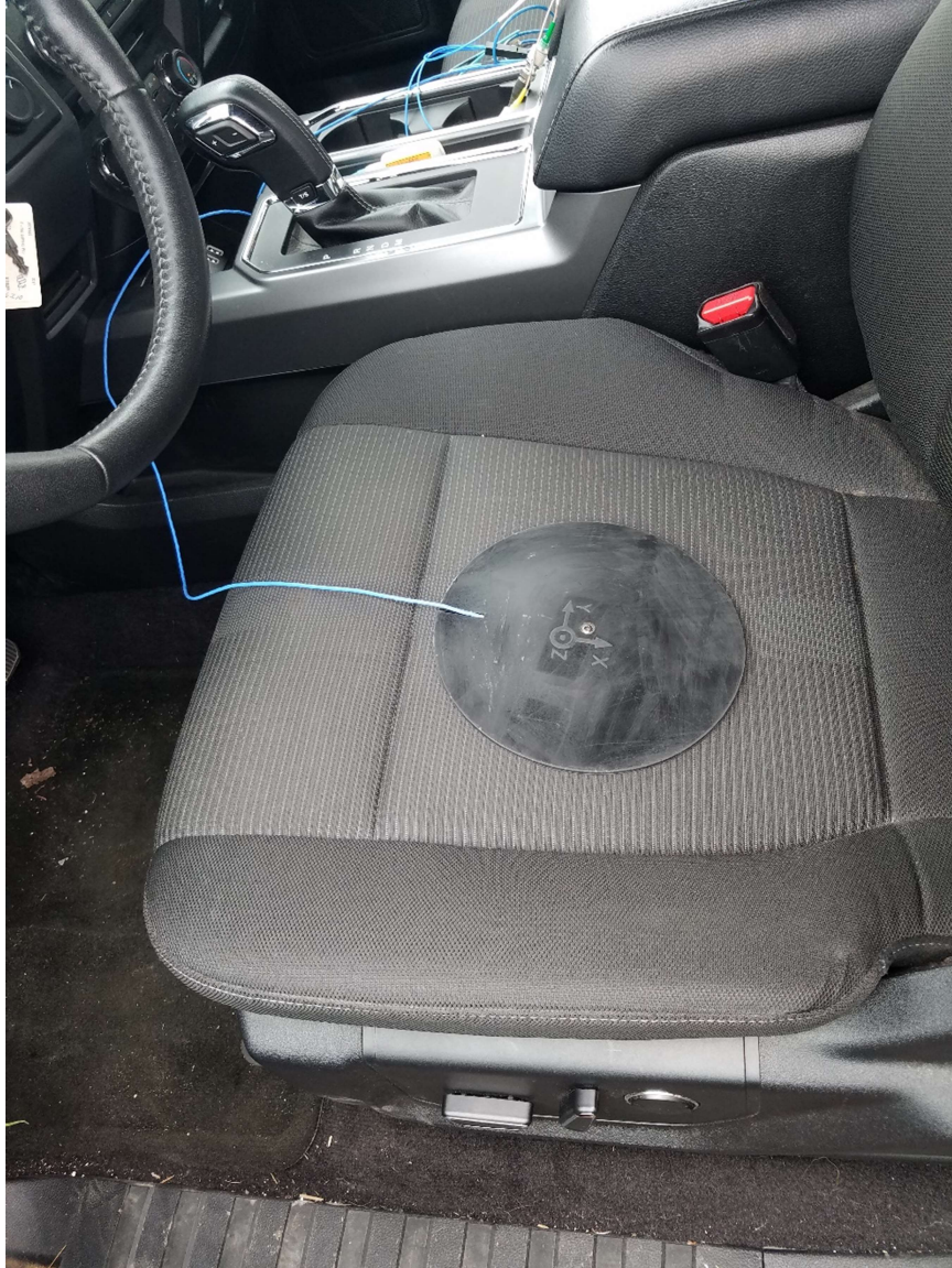
Figure 117: Seat Pad Accelerometer Mounting
