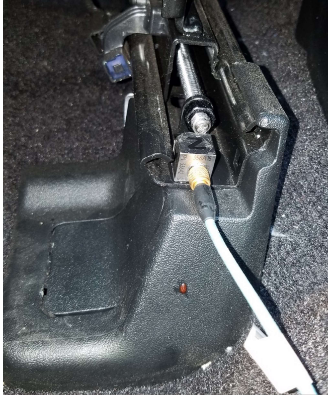
Figure 116: Seat Track Accelerometer Mounting
