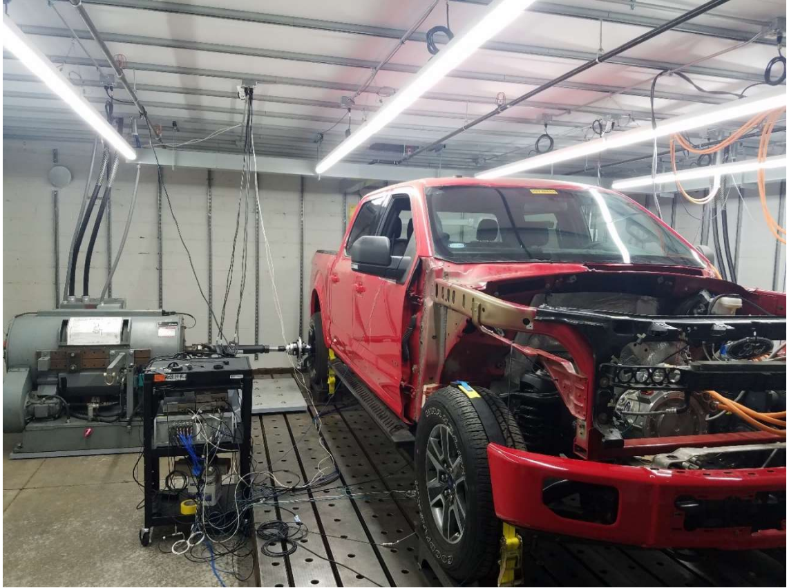
Figure 108: Passenger Side View of Laboratory Test Vehicle on Dyno
