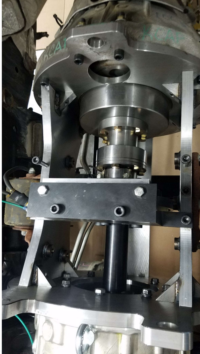
Figure 109: Top Down View of Cradle Assembly Coupled to the Transmission Bellhousing (top) and eMotor (bottom) Complete with Shafting and Torque Telemetry Mounting
