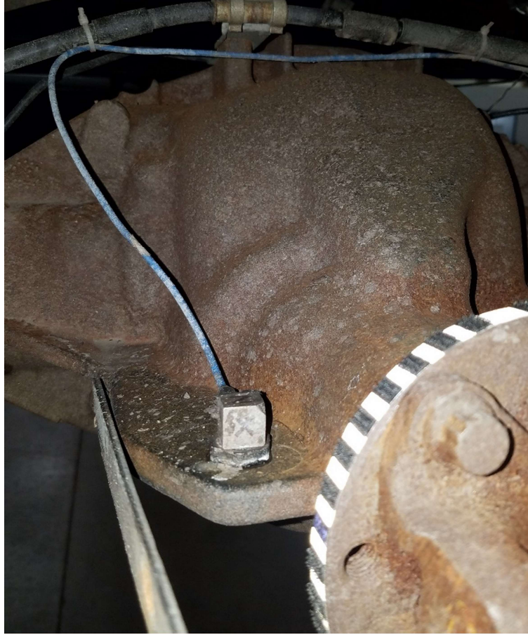
Figure 113: Differential Accelerometer Mounting
