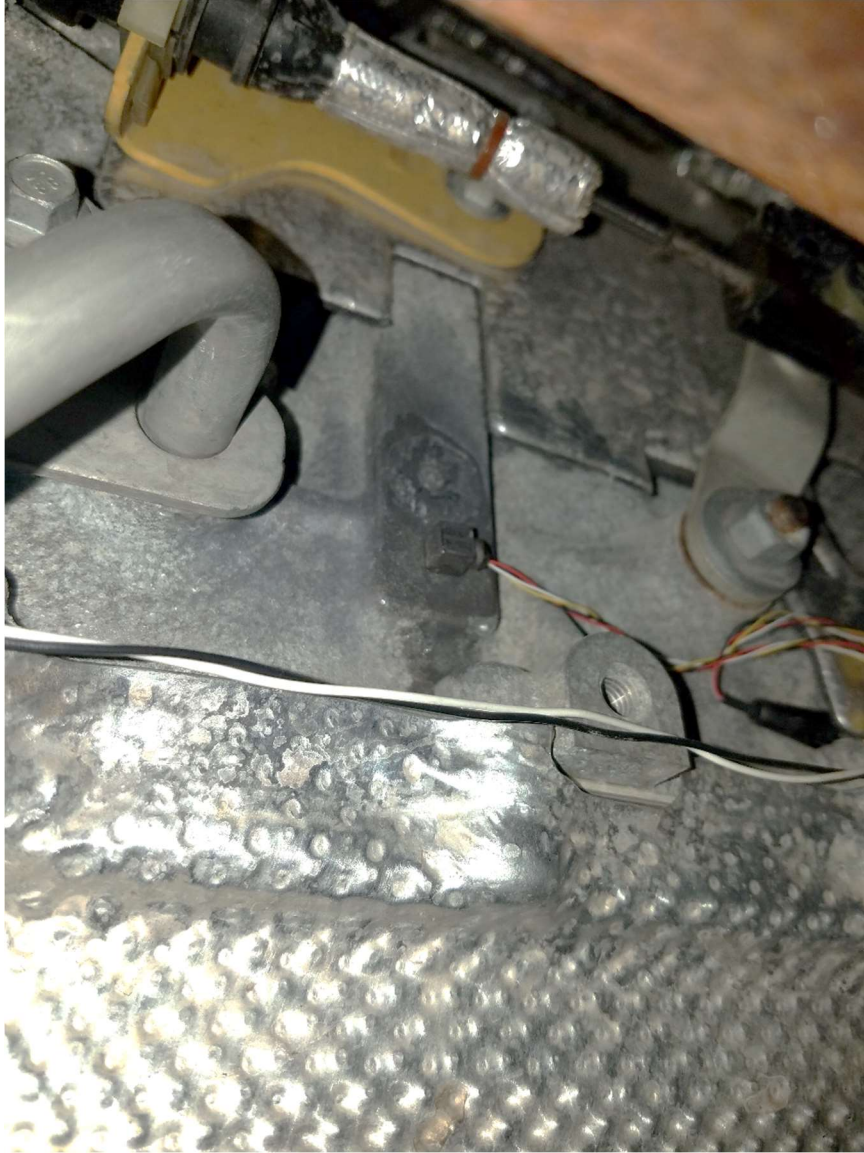
Figure 114: Transmission Accelerometer Mounting
