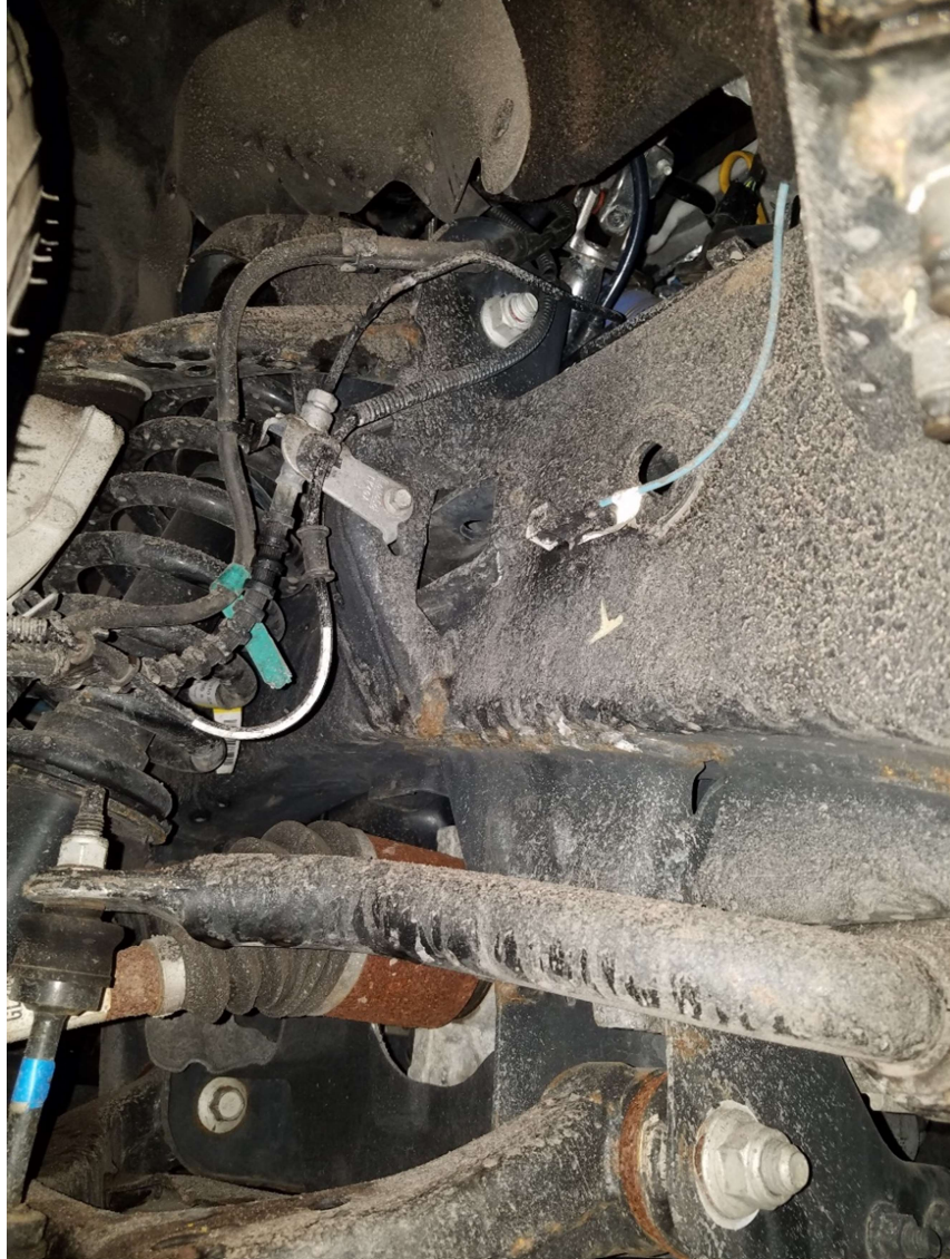
Figure 115: Chassis Accelerometer Mounting
